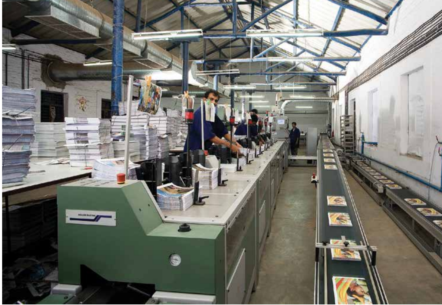
Right: Muller Martini Acoro A5 automated perfect binding machine
